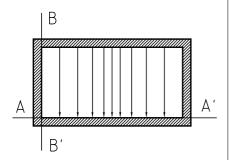
From these considerations it can be understood that at a given frequency a minimum size of one side of the rectangular waveguide is required to have the lowest order mode above cutoff. This minimum size is half the wavelength of the electromagnetic power. For a frequency of 2.45 GHz this minimum size is 61.2 mm. By means of the axial wavenumber a waveguide wavelength can be calculated to be:
