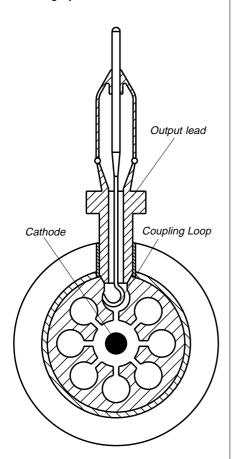
Cross Section of a Magnetron
